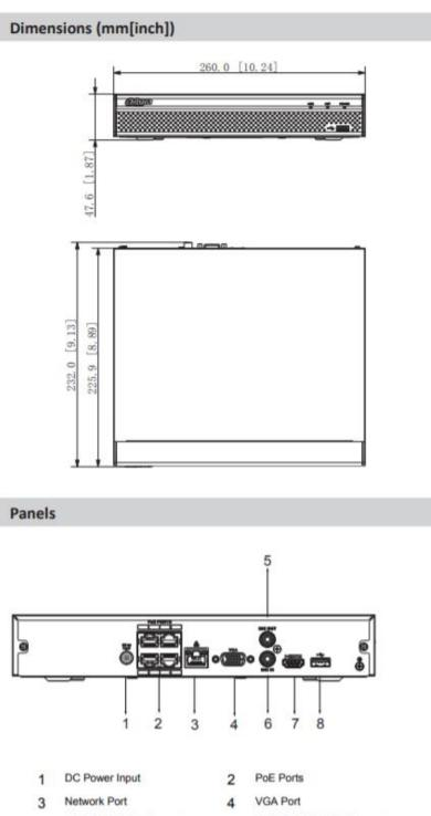
AUDIO IN, RCA Connector 6 AUDIO OUT, RCA Connector
