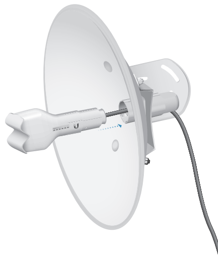
Single Cable Connection with InnerFeed Technology
